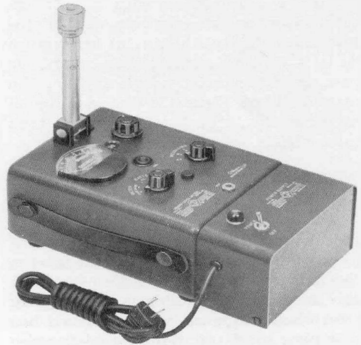
Figure 8. View of Sound-Level Meter with A-C Power Supply attached.
