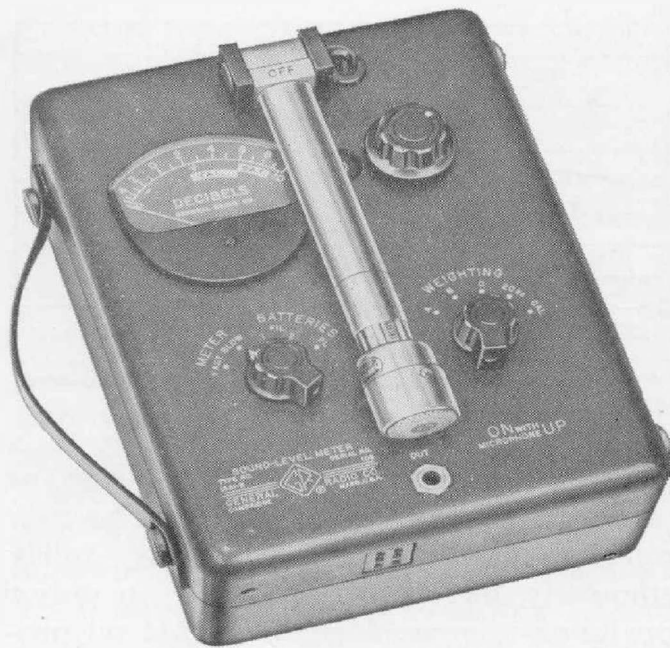
Figure 1. Panel view of the Sound-Level Meter, with microphone folded down in OFF position. In operating position, microphone can be either erect, as shown on front cover, or extending outward from case.
